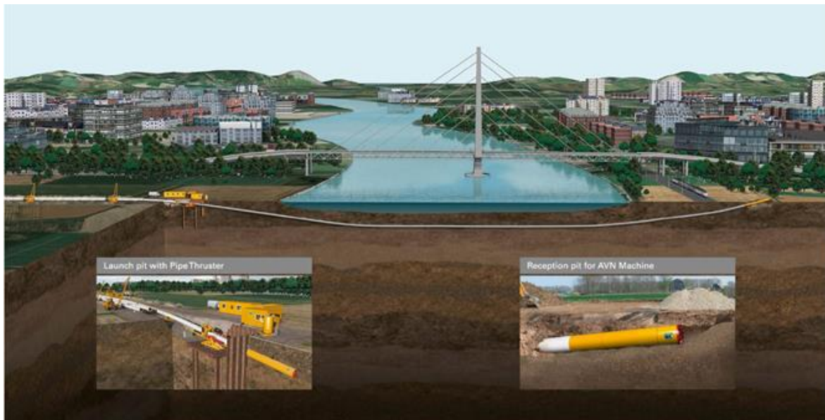
Figure 5: A sample of a standard Direct Pipe® Operation
