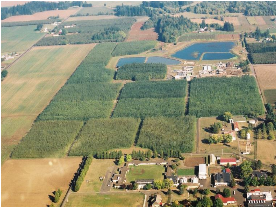
Figure 4. Poplar plantation in Woodburn, Oregon. The woodlands are irrigated with effluent from the lagoon treatment system.
