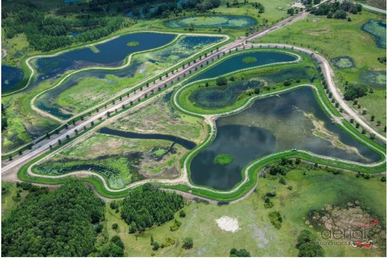
Figure 1. 4G groundwater recharge wetlands, Pasco County, Florida. Wetlands receive 19 MLD of secondary effluent to percolate downward to water table. Total nitrogen, which is almost all nitrate, is reduced to background concentrations by natural means as it passes through wetland soils.
