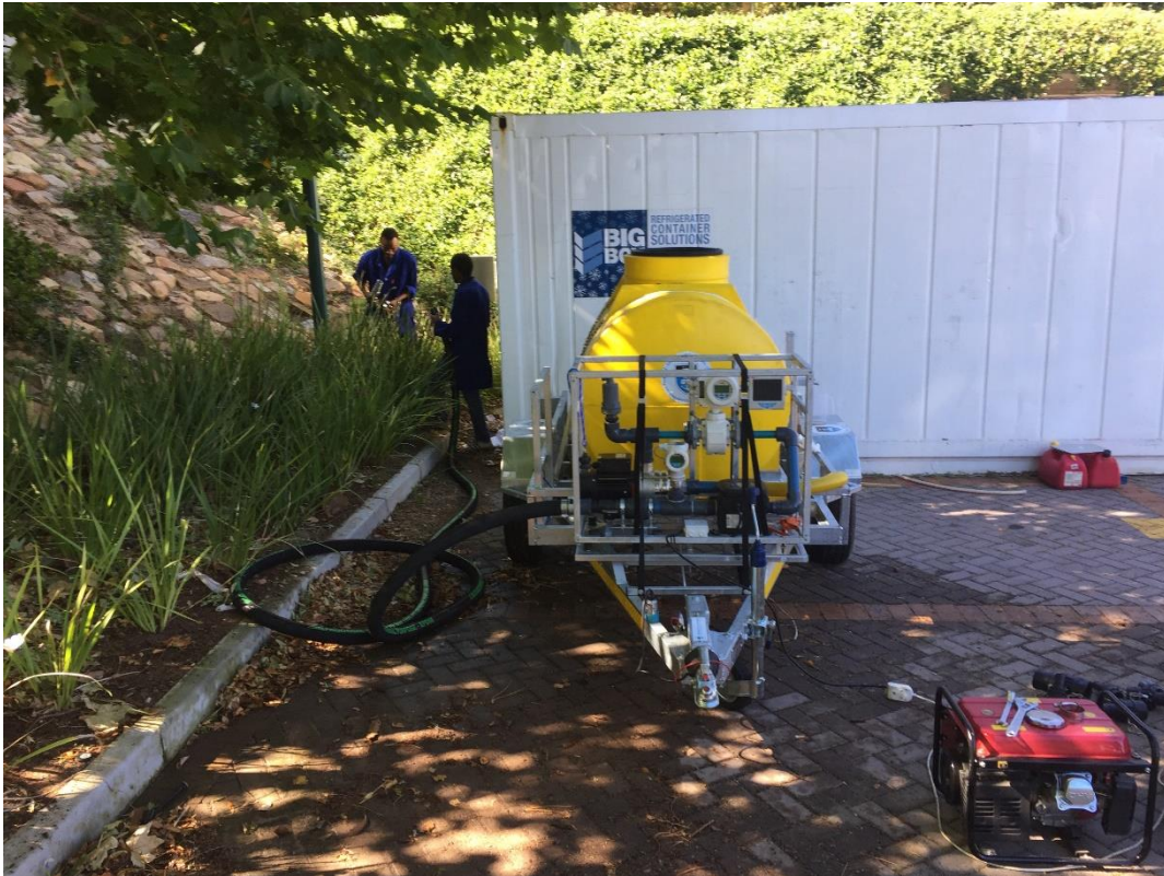
Figure 1: Pipe condition assessment equipment
