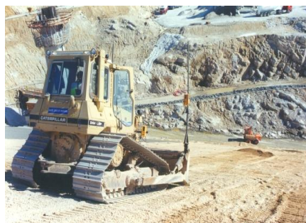
Figure 3: Laser- equipped dozer pushing limesto
