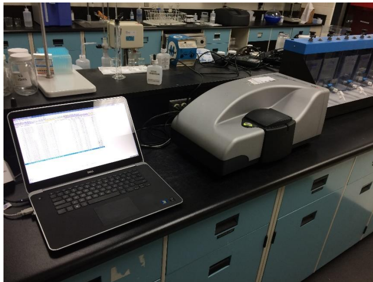
Figure 10: Malvern Zetasizer and jar testing equipment
