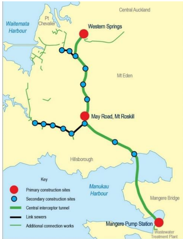
Figure 2: Central Interceptor Project Overview
