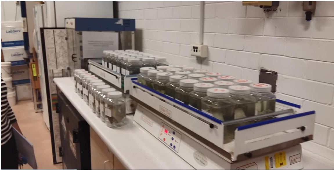
Photograph 5: Acid Bath Immersion Test Rig at the University of Sydney
