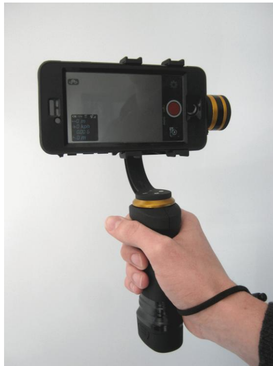
Photograph 2: Setup of geo-referenced video camera on handheld stabilising gimbal.
