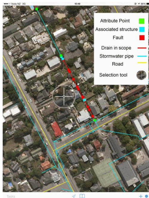
Figure 2: Screenshot of tablet map application showing GIS data and data points captured in the field.
