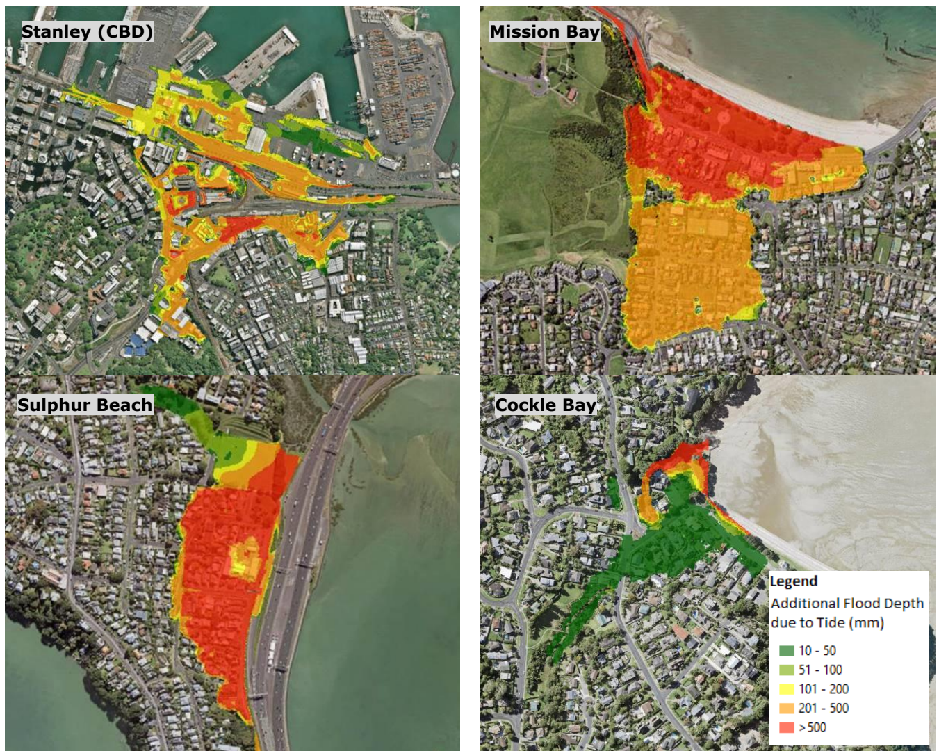
Figure 10: Increase in 100yr Flood Depth with 100yr Storm Tide+1m SLR compared to No Tide Scenario (Scenario 4 minus Scenario 2)
