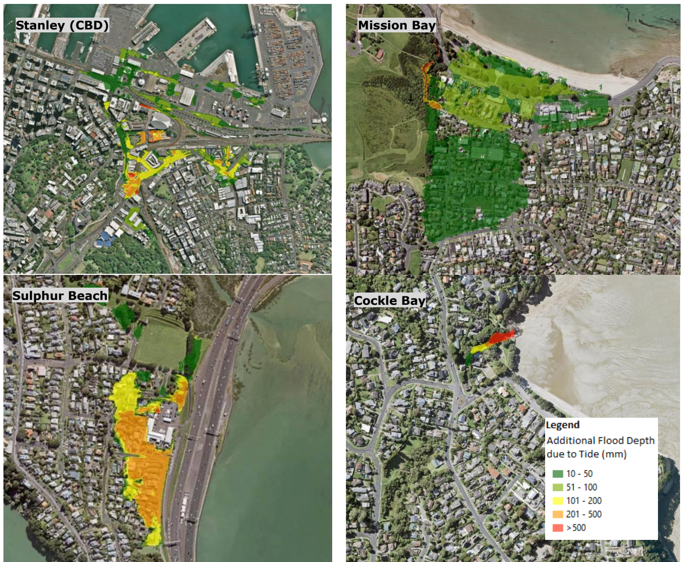
Figure 9: Increase in 100yr Flood Depth with 100yr Storm Tide compared to No Tide Scenario (Scenario 1 minus Scenario 2)
