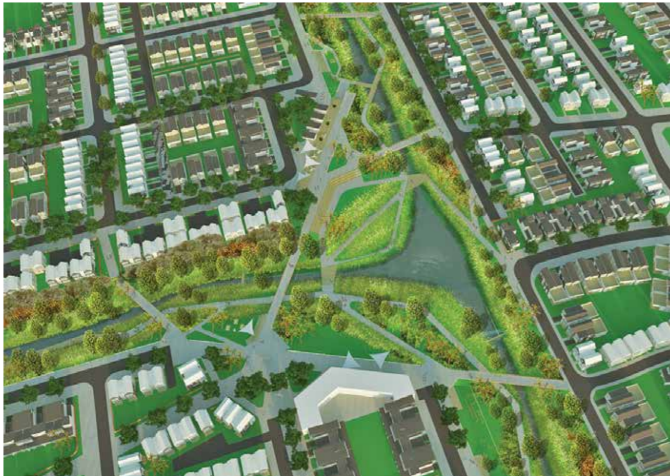
Above: Stage One of the Awakeri Wetlands Project, costing some $45 million, is focused on construction of a t-shaped, 2.3-kilometre-long wetland stormwater channel running from Grove to Cosgrave to Walters Roads which will enable more new housing developments in this area. Below: Awakeri Wetlands Project opening the way to eco-friendly communities.
