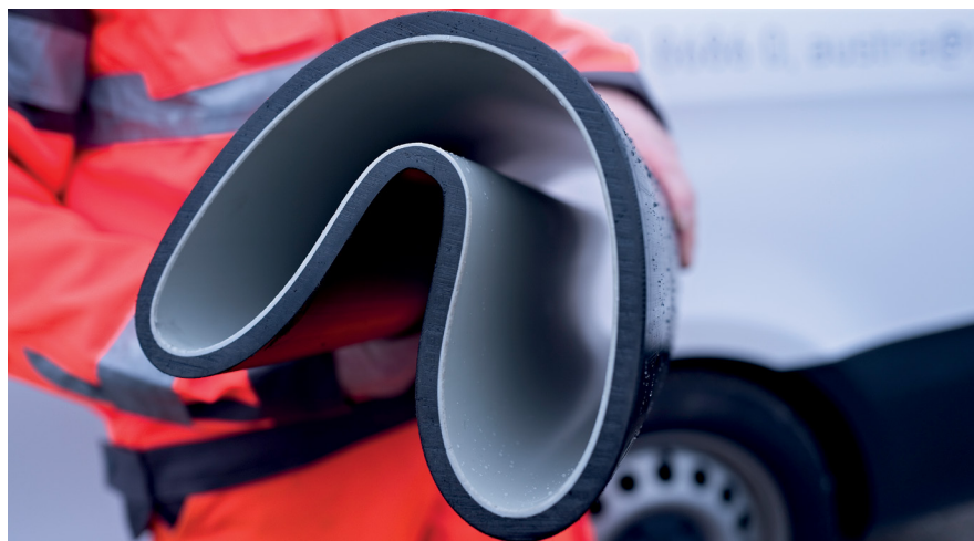
When relining without an annular space, a folded and therefore reduced PE pipe string, the so-called AGRU SureFIT liner, will be pulled into the old pipe. Pipes and entire tunnels with cross sections of more than 1 metre in diameter are thermo-plastically lined with AGRUSAFE concrete protection liners.
