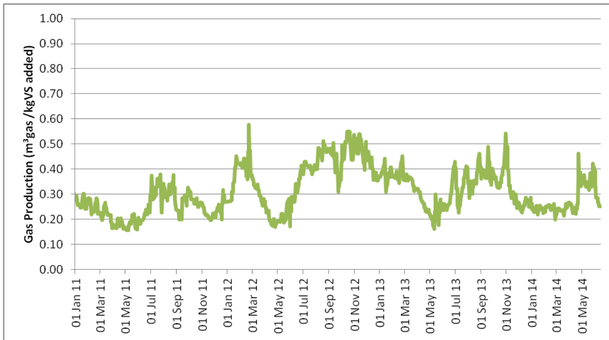
Figure 9 Specific Gas Production at the Pukete plant, Please note that recuperative thickening was practiced between March 2013 and June 2014
