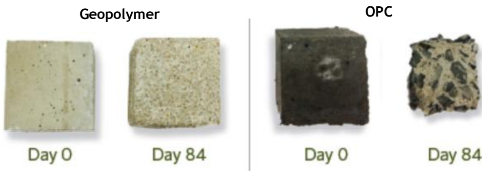
Figure 7: Image of cubes before and after soaking in 7% H 2 SO 4
