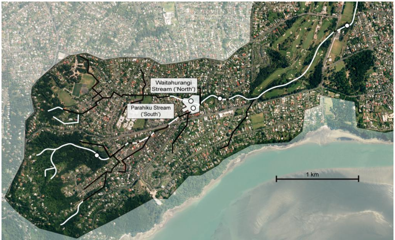
Figure 1: Map showing the location of the daylighted stream reaches. Sampling locations are shown by white circles. The opaque polygon shows the location of the La Rosa reserve and the sampling locations within this polygon represent the daylighted reaches. In the wider catchment, open channels (un-piped) are indicated by white lines and piped channel is shown as black lines.
