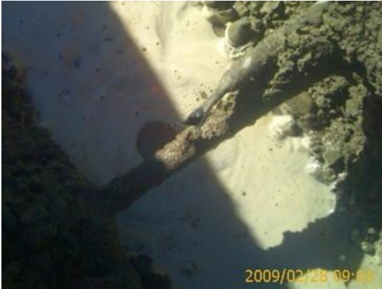
Figure 13. Tensile failure of black PE pipe without gross extension.
