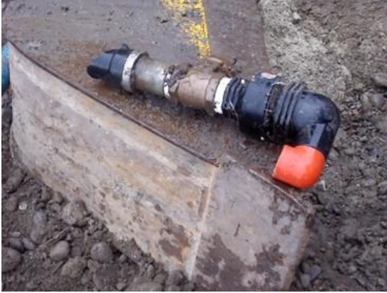
Figure 3. Fractured injection moulded compression fitting elbow showing mixed materials (Citycare).
