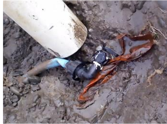
F14. Severe bending in PE80 service pipe. Despite being effectively closed off, the pipe has not failed.
