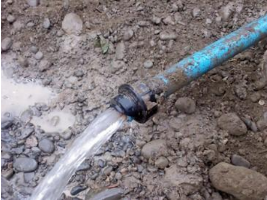
Figure 9. Leaking compression fitting assembly (Citycare)
