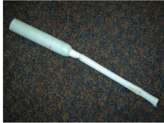
F14. Severe bending in PE80 service pipe. Despite being effectively closed off, the pipe has not failed.
