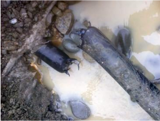
Figure 13. Tensile failure of black PE pipe without gross extension.
