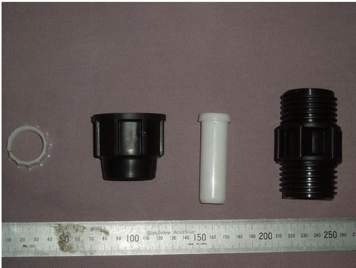
Figure 15. Components of a Plasson DN 25 straight coupler. From left: grip ring, Collar, insert, fitting body.
