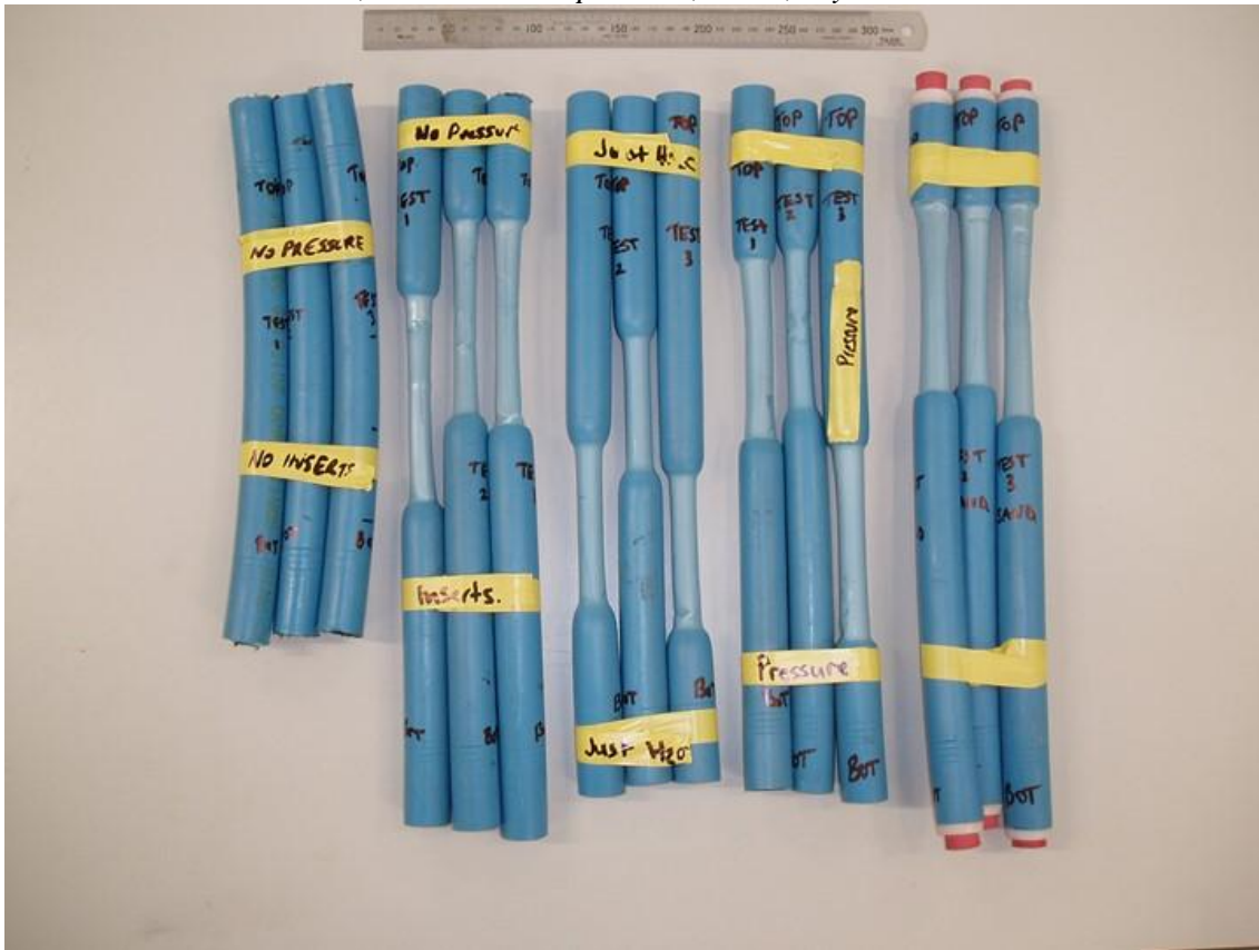
Figure 16. DN25 PE80 service pipe assemblies after testing. The top as tested is next to the 300 mm ruler. From the left: No insert, empty pipe; Insert, empty pipe; Insert, water but no pressure; Insert, water at mains pressure; Insert, dry beach sand.
