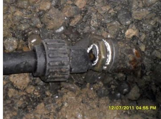
Figure 10. Damaged compression fitting assembly (Citycare)
