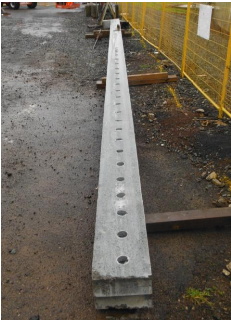
Figures 4A and 4B - Saw Cut Removed Stitch Showing Duct Deformities
