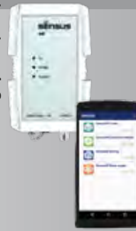
Automatic Meter Reading System (AMR)
