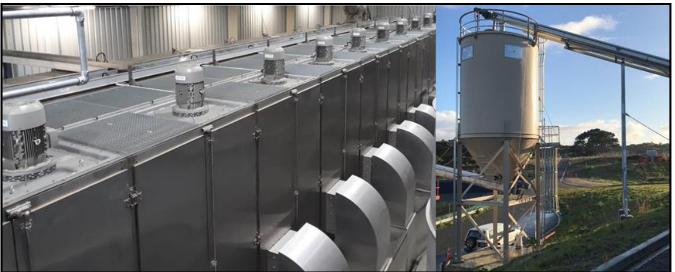
Photograph 13/14: Thermal Sludge Dryer (left), Dried Sludge Storage/Outloading (right)
