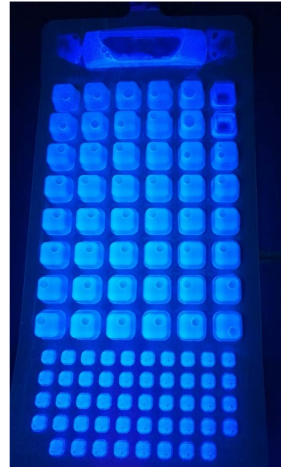
Colilert and Pseudalert Quanti-trays under the UV light
