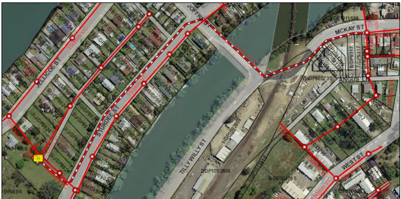
Photograph 2: Red and white, denotes Sewer Rising Main.
