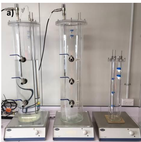
Photo 3: Scale up gear: a) 15 L bioreactors alongside a 3 L bioreactor; b) The new Watercare's Wastewater Innovation Centre, home of the anammox bioreactors.
