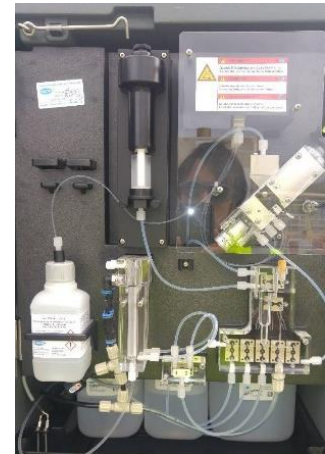
Figure 6: AMTAX unit internals
