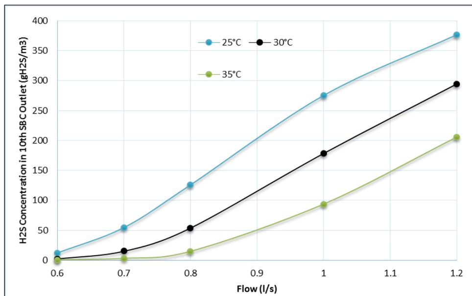
At higher (summer) temperatures the bioreactor operates more effectively and the H<sub>2</sub>S consent limit can almost be met at a flowrate of 0.9m/s. Conversely at the lower (winter) temperature condition, the bioreactor flow would need to be reduced to meet consent requirements.
