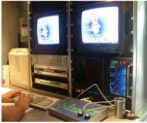
Figure 11: Control panel for CCTV inspection
