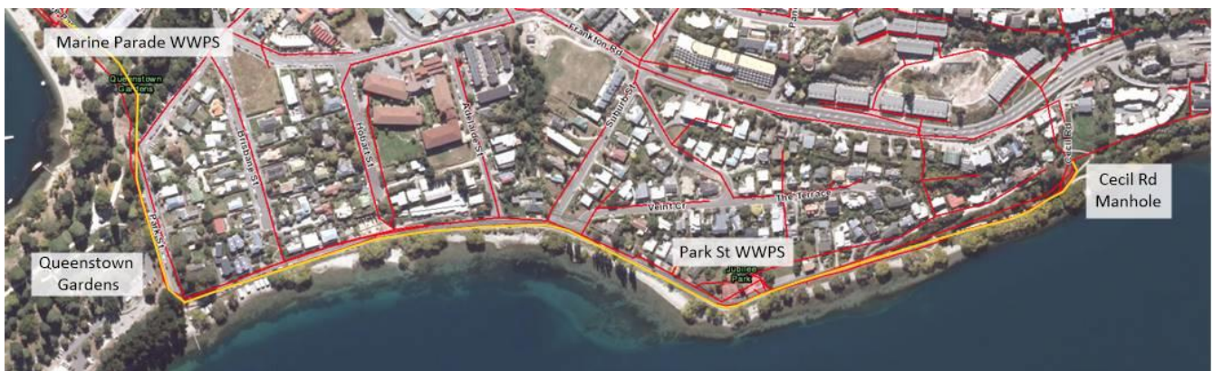
Figure 3: General arrangement of rising main alignment
