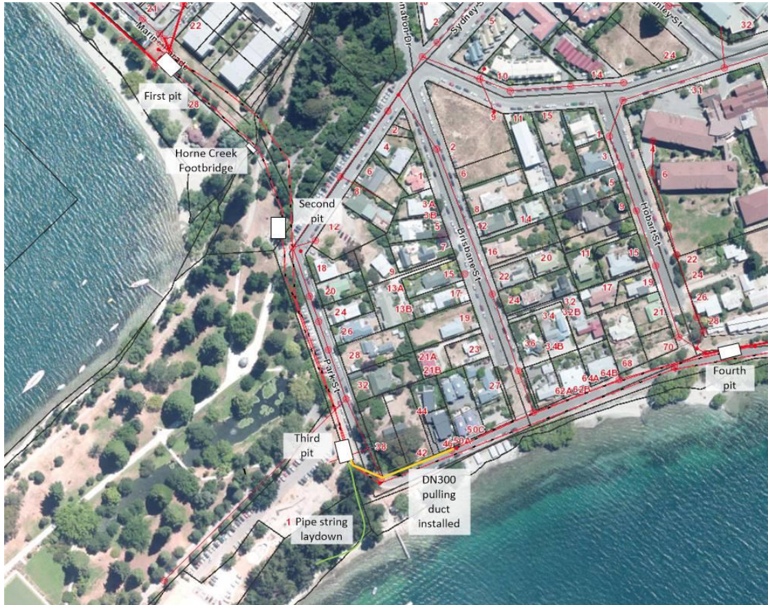
Figure 9: Overview of works through the Botanic Gardens. Minimal impact on public amenity, environmental and historical values through slip-lining. Adjusting the plan to suit found conditions avoided disruption to Park Street traffic
