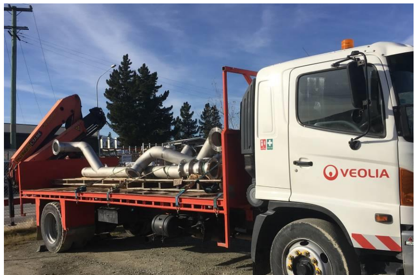
Figure 6: Replacement risers ready for transport to site
