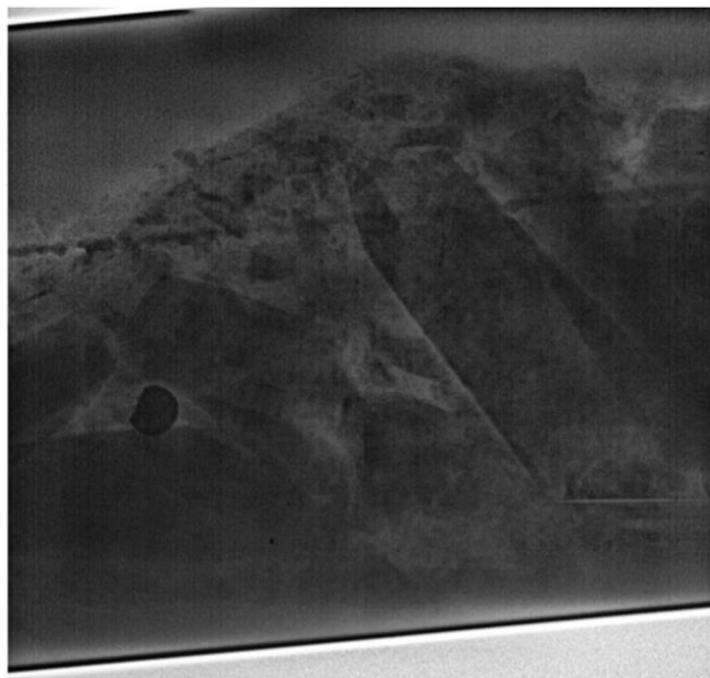
Figure 8 An X-ray image of a 150mm pipe without water and with sediment.
