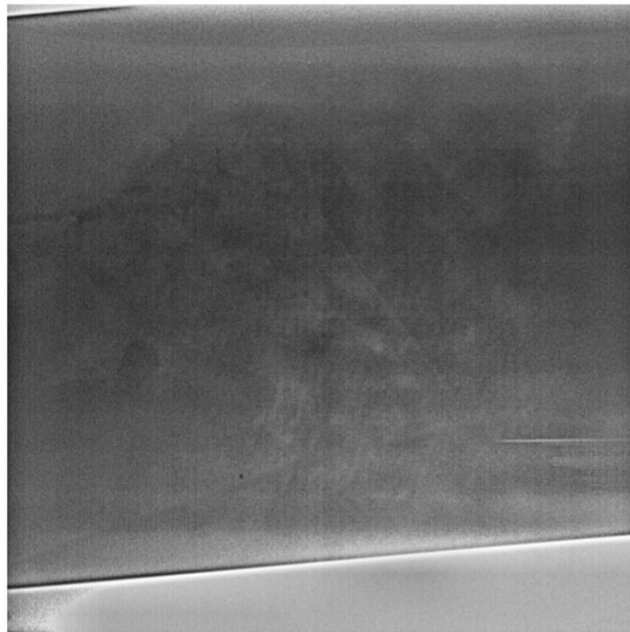
Figure 7 X-ray image of a 150mm pipe with water and sediment.
