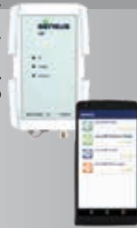
Automatic Meter Reading System (AMR)
