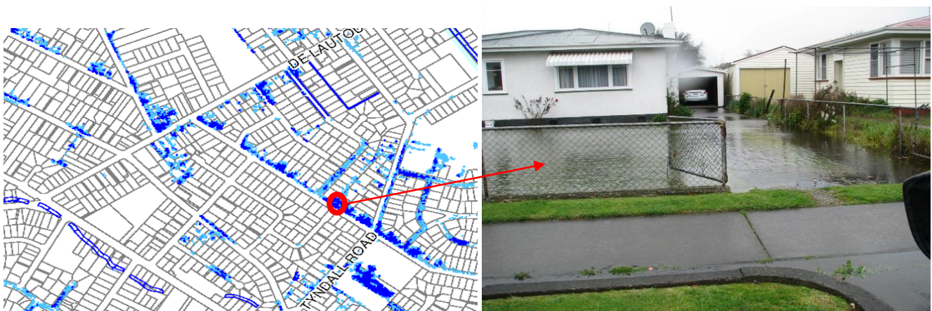
Figure 4 – Outputs from catchment modelling of the Kaiti catchment, Gisborne (showing that overland flow is trapped on parcels as roads are higher than surrounding area) and event photo from Sept 2015.
