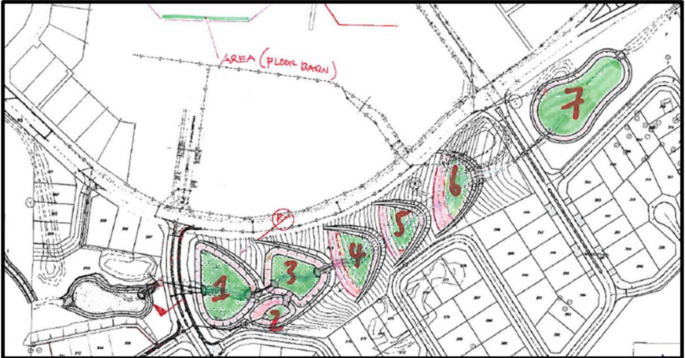
Figure 2 - Original engineering concept to manage flooding
