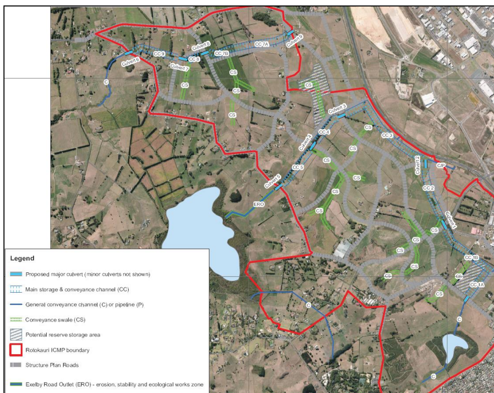
Figure 2: Rotokauri Stormwater Conveyance Infrastructure. Wetlands are located within main storage and conveyance channel in blue (CC), which is located in a green corridor. 2018 Stormwater Conference
