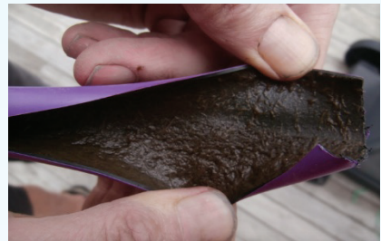
Drip line needs flushing
