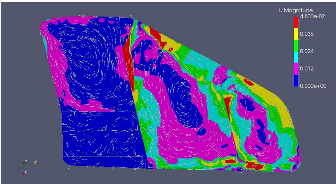
Figure 7: Bottom velocity distribution model 3
