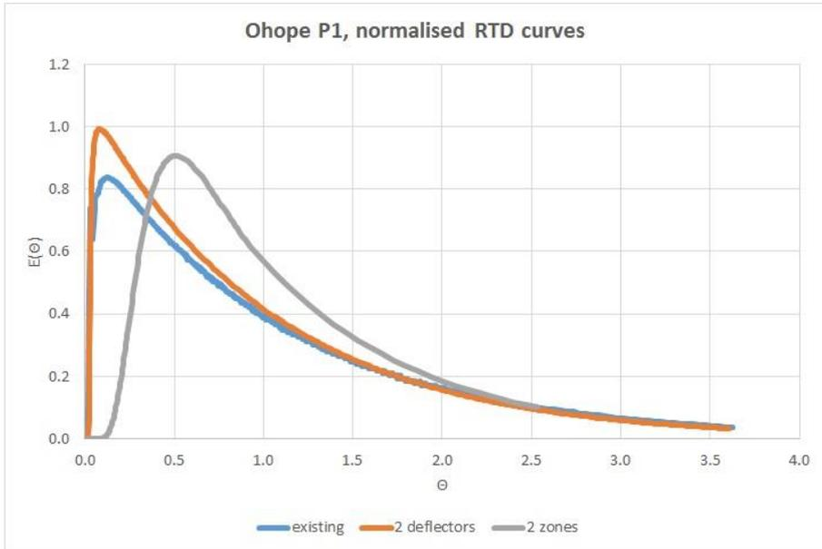
Figure 9: Comparison of RTD curves, 3 models
