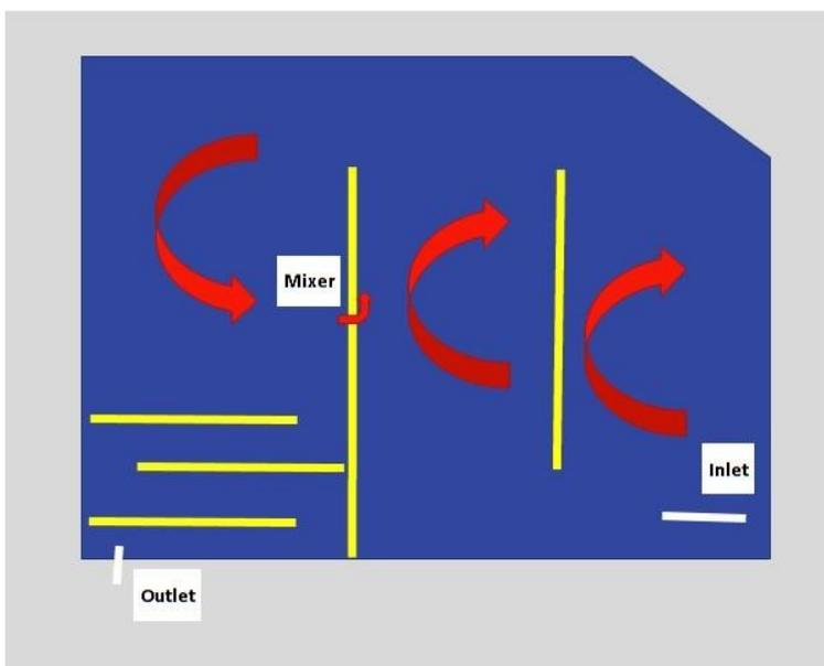
Figure 4: Schematic model 3, pond area split into 2 zones (mixing and retention)
