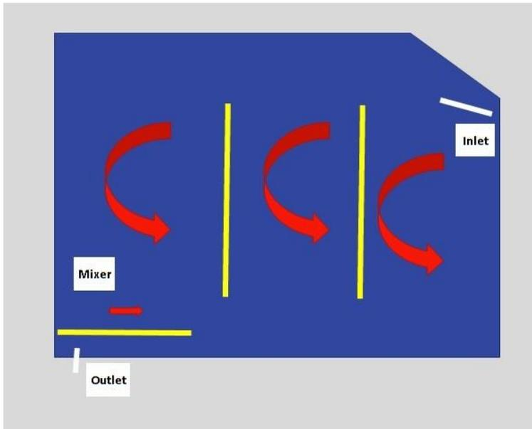
Figure 3: Schematic model 2, using 2 baffles to separate 3 zones
