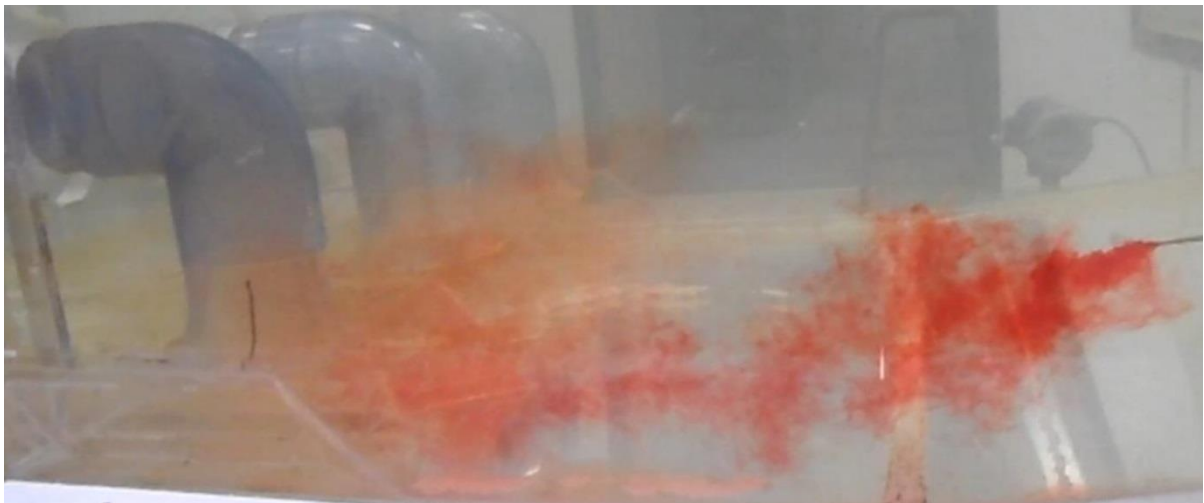
Figure 14: Case 4 – Smooth Streamline into Suction Bell (Dye visualization)
