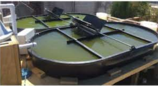
High Rate Algal Ponds (HRAPs) for sunlight disinfection, organic compound (e.g. BOD 5 ) and nutrient removal
