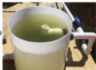
Algal Harvester (AH) for algal solids removal from the HRAP effluent
