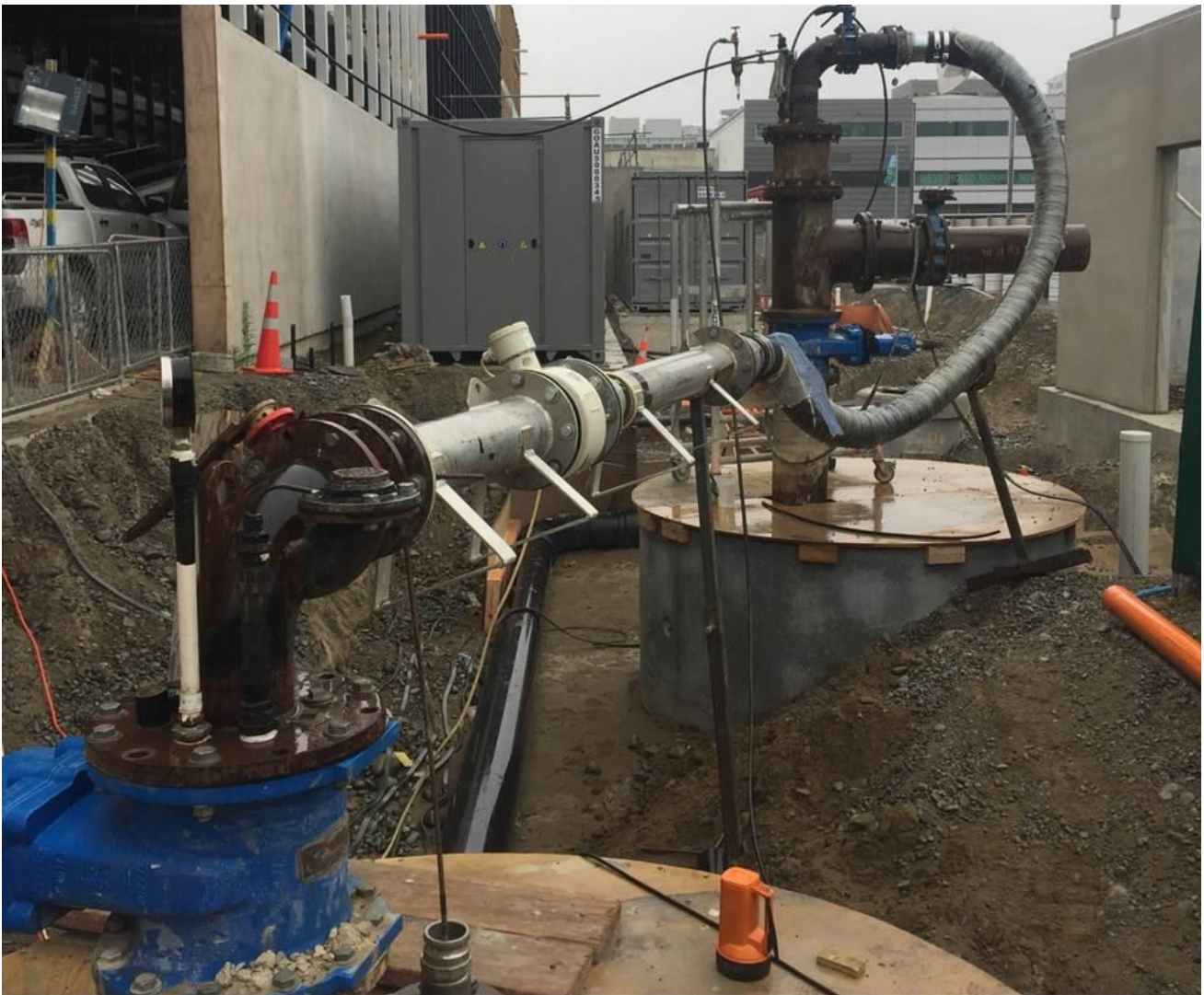
Photograph 1: Pumping test of an abstraction well (left) and reInjection well (right) to determine well hydraulic performance (photo courtesy of McMillan Drilling)
