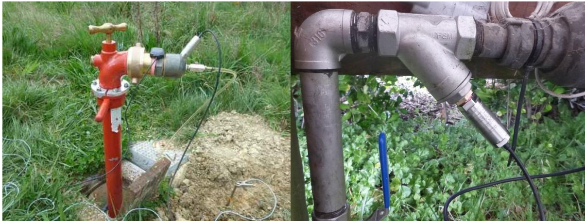
Figure 2: Transient measurement stations.
