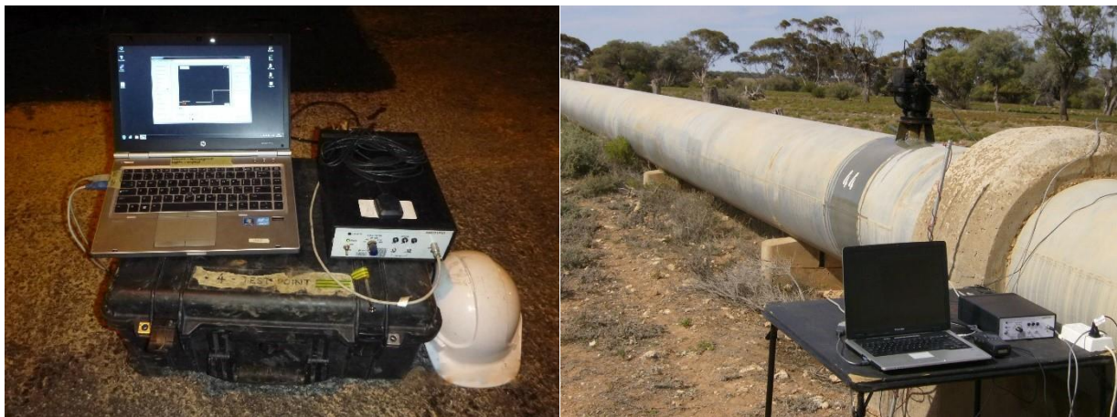
Figure 3: Transient data acquisition system set up.
