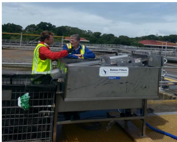
Figure 3: Early Pilot Trails of the baleen Filter at New Plymouth WWTP. Courtesy: Bioholdings New Zealand Ltd.
