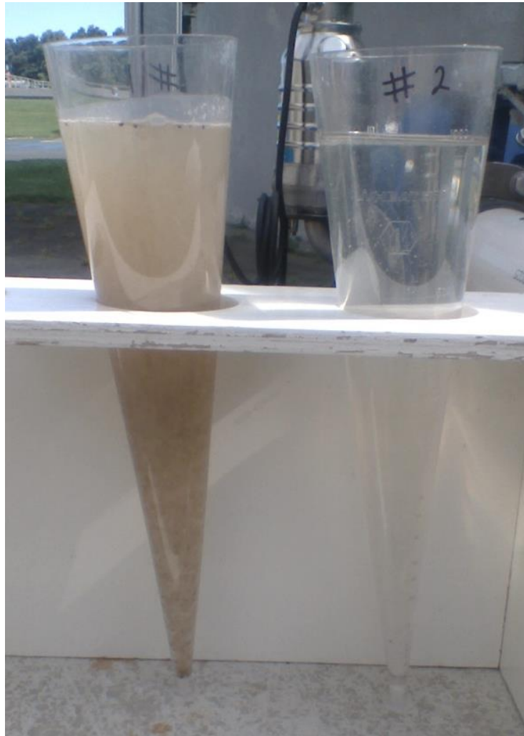
Figure 6: Cone test of scum feed to Baleen Filter, and resulting filtrate (right).
