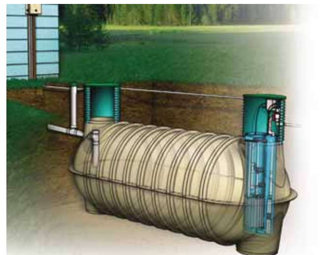
Below – Both pumped (STEP) and gravity-discharge (STEG) lots can be connected to the same small diameter effluent sewer system, Bottom – Orenco ProSTEP® on lot pumping package inside a 4,000 litre fibreglass tank
