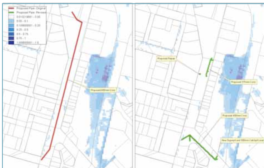
Figure 2 – Predicted surface flooding in shopping precinct
