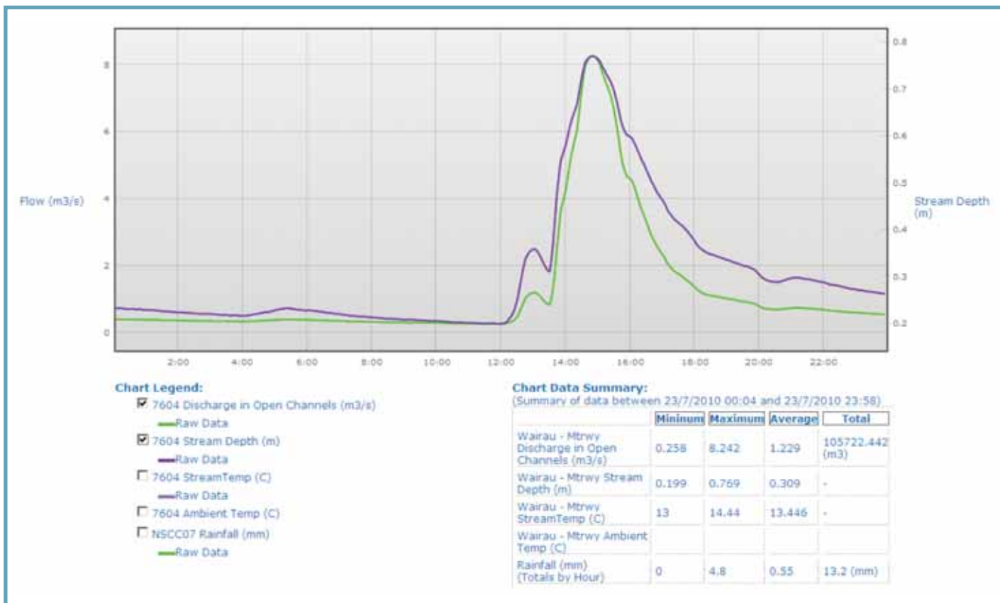
Figure 4 – Stage and discharge data presented via web-based access
