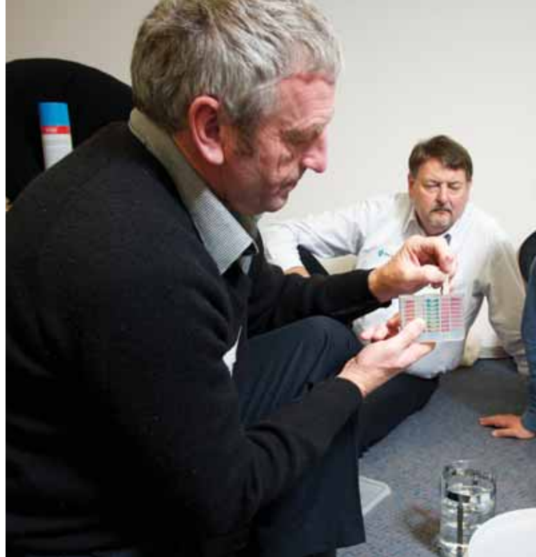
Using a chlorine comparator kit (left to right) – Geoff Horler – Hurunui District Council, Martyn Simpson – Water Industry Training and Len Williams – Castlecorp
