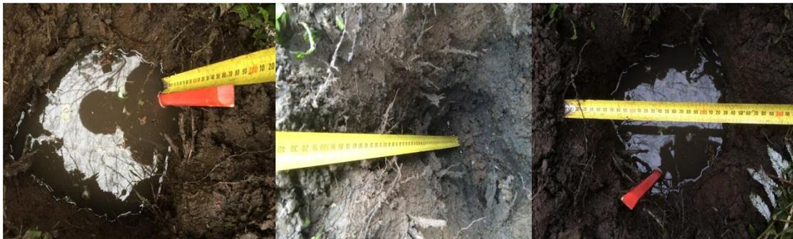
*Figure 2: Excavated holes for testing hydraulic conductivity of the soil.*
