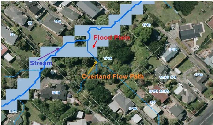
Figure 3: An aerial view of the site showing the overland flow path and the stream at the back of the site.
