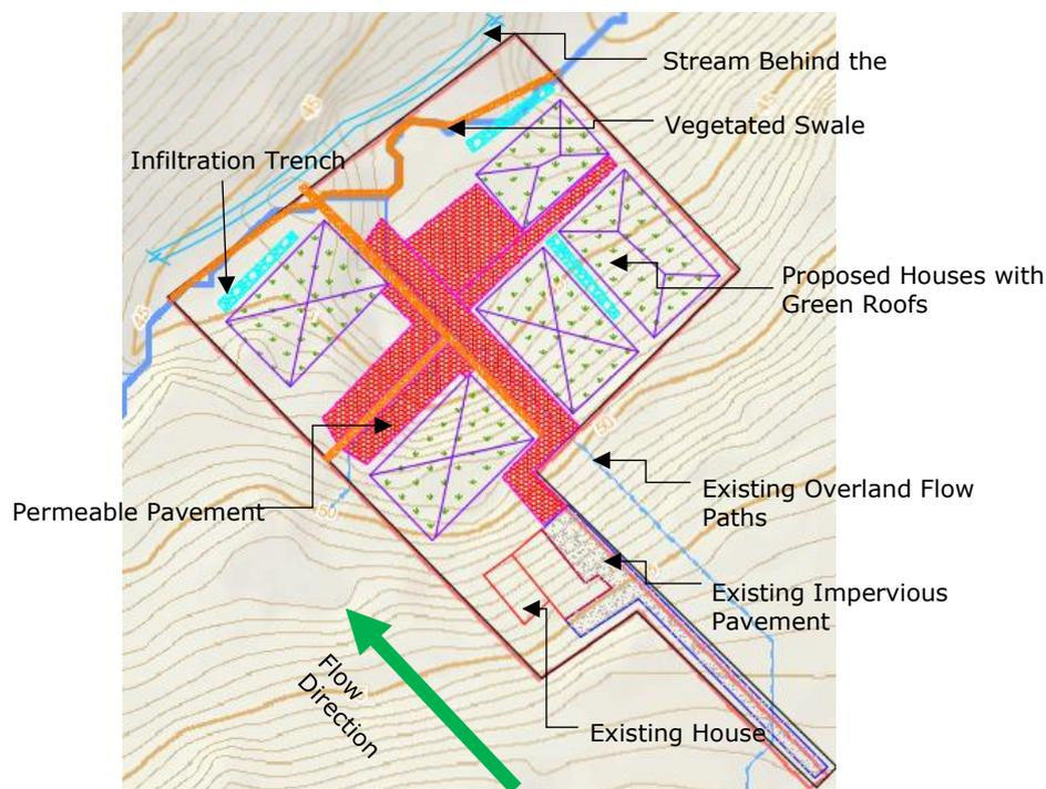
Figure 4. A plan view of the proposed LID System (Option 2).
