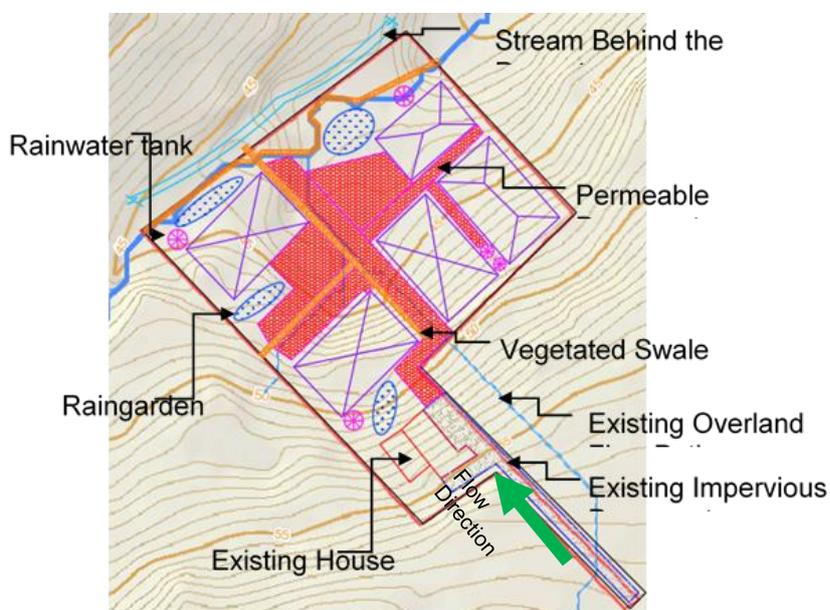
Figure 5: A plan view of the proposed HSMS (Option 3).
