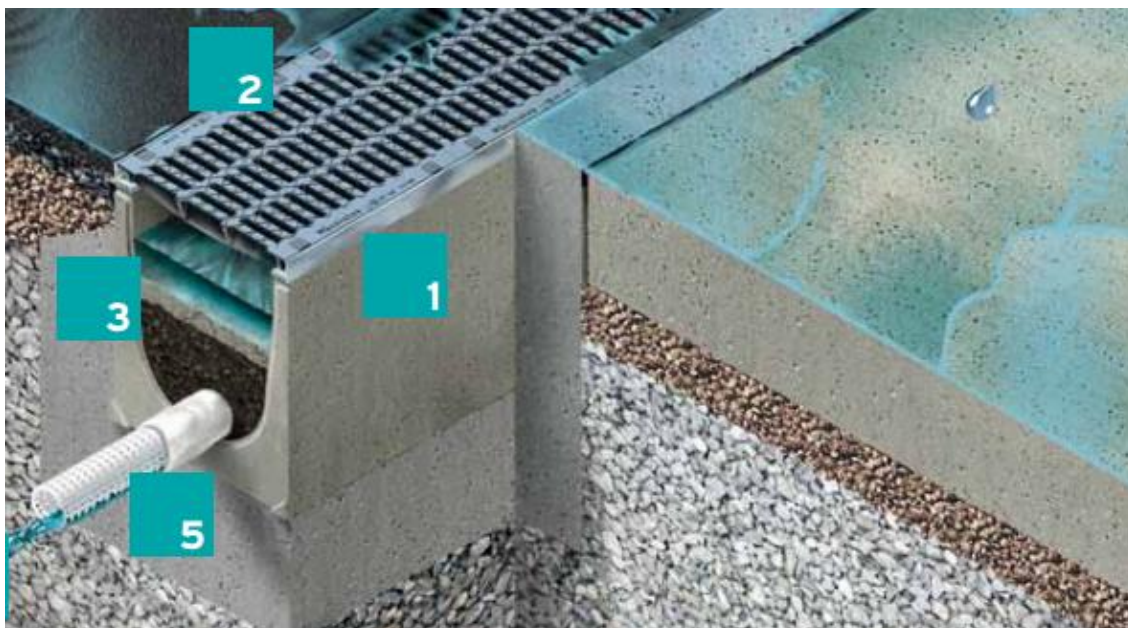
Figure 2: Drainfix Clean device. Key: 1 = drainage channel; 2 = channel grating; 3 = filter media; 5 = treated runoff drainage collection pipe (image courtesy of Hauraton)
