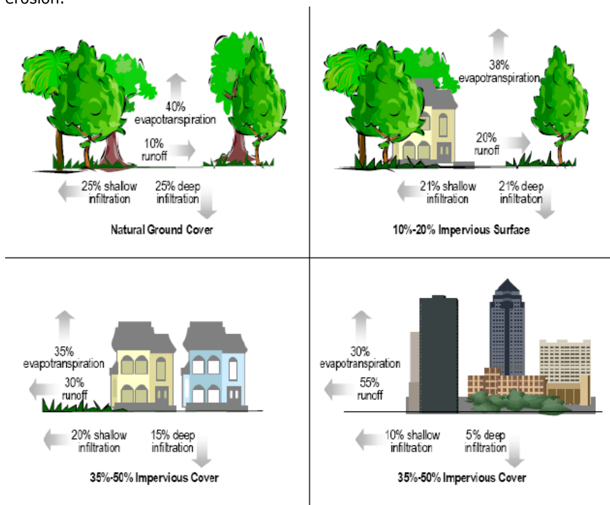
Figure 1: Impacts of Urbanisation on the water cycle (Source: United States Environmental Protection Agency, 2005)
