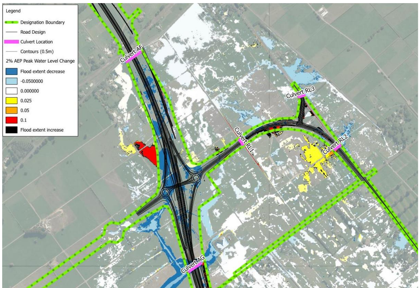
Figure 9: Example output for Waikato Expressway culvert design, showing areas exceeding the 50mm flood afflux requirement. Note this is a draft iteration for illustration purposes only and not the final result.
