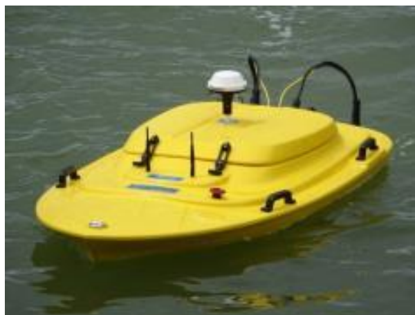
Photograph 1: The Q-boat set up with the propellers and GPS, ready to survey.
