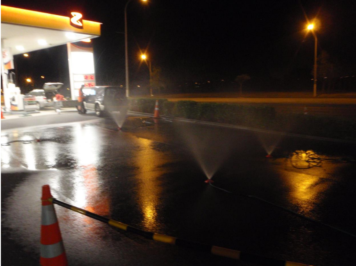
Figure 1: Synthetic rainfall being applied across a non-forecourt catchment.
