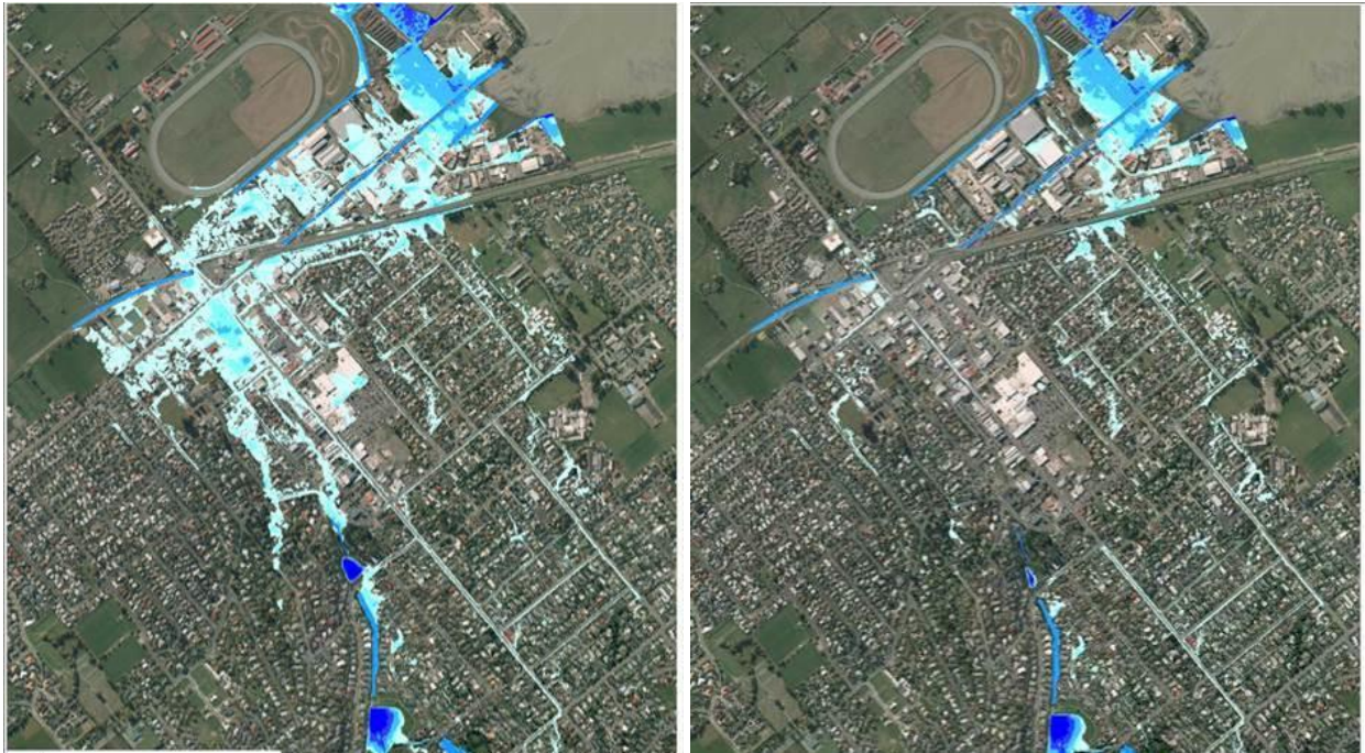
Figure 9: 100-year flood model of current system (left) after preferred solution (right)
