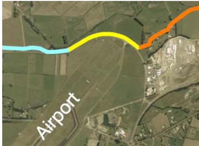
Figure 7: Christchurch Airport Secondary Stopbank Gap (Yellow line represents new stopbank required to fill gap in secondary stopbank line)
