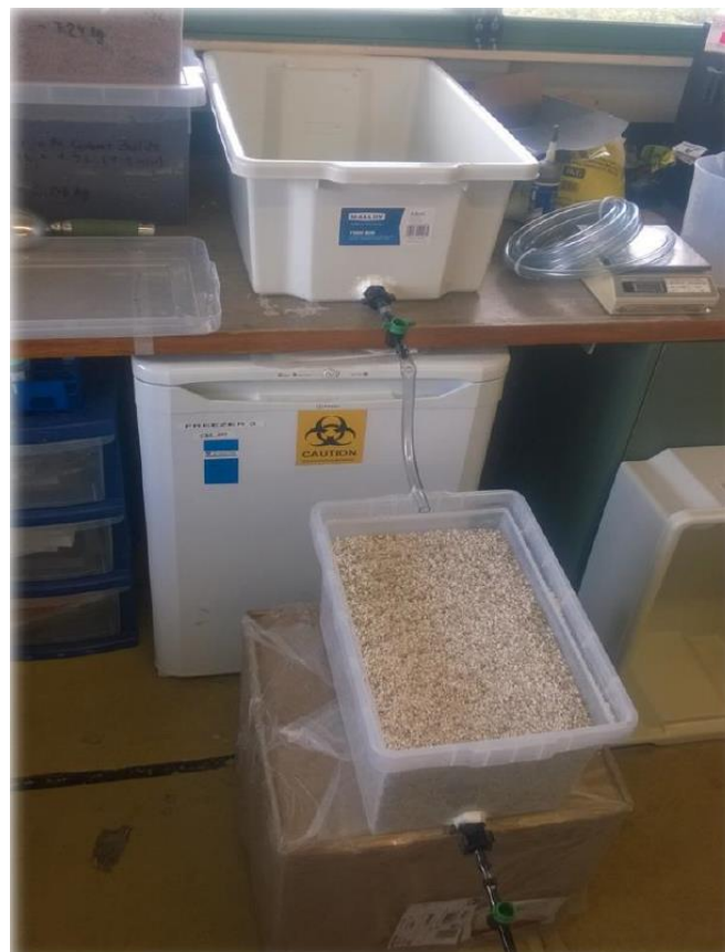
Figure 9: Laboratory bench-scale set up for stormwater runoff treatment
