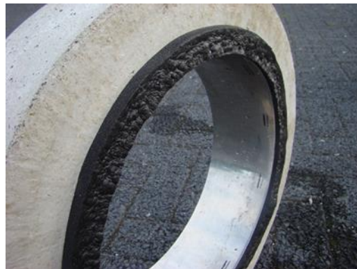
Photo 3: Indentations in soft foam from being placed on the paver surface to form a seal.
