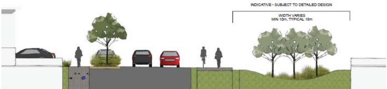
Figure 2 Huapai Triangle road cross section showing the large overland flow path/swale v .
